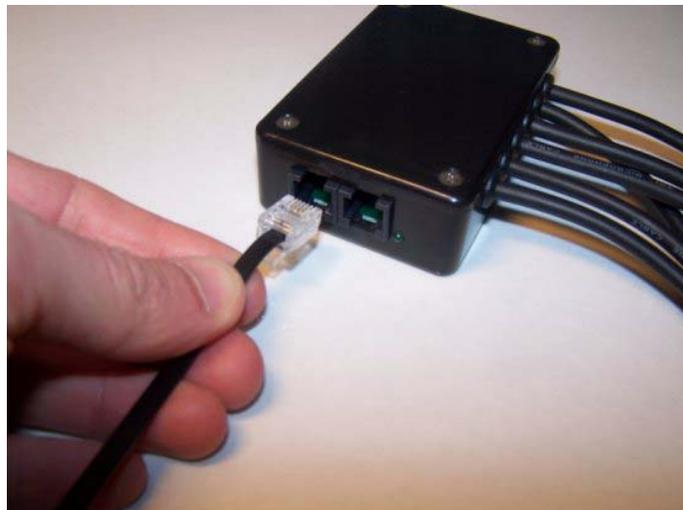
The modules are connected one to another using RJ11 wires. Check the proper « click » sound when inserting the RJ11 connectors in the plugs.
